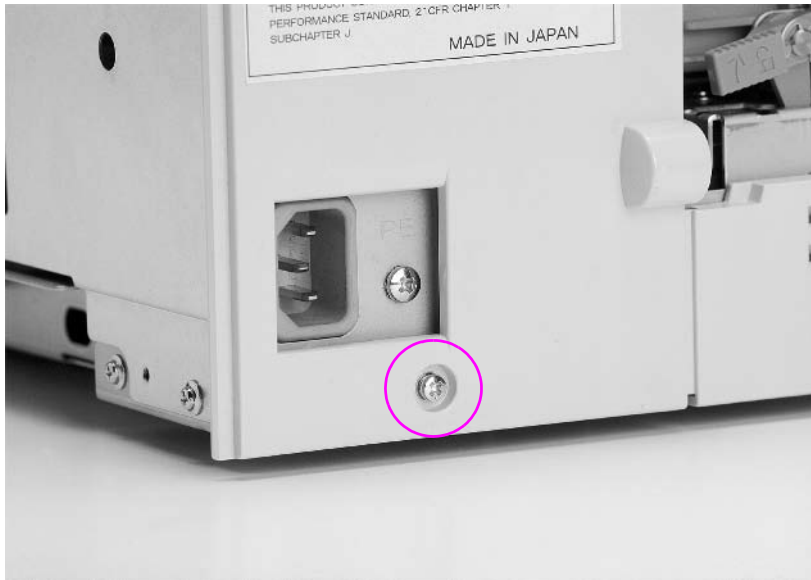
Figure 6-6 Right rear cover removal and replacement
