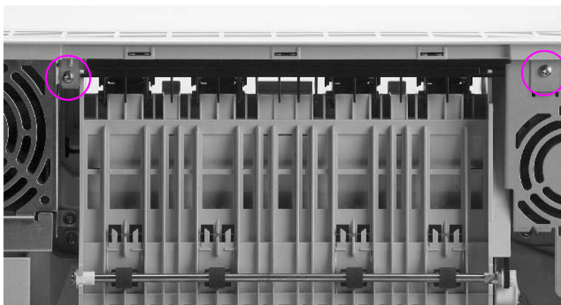
Figure 6-2 Top cover removal and replacement (rear view of printer)
