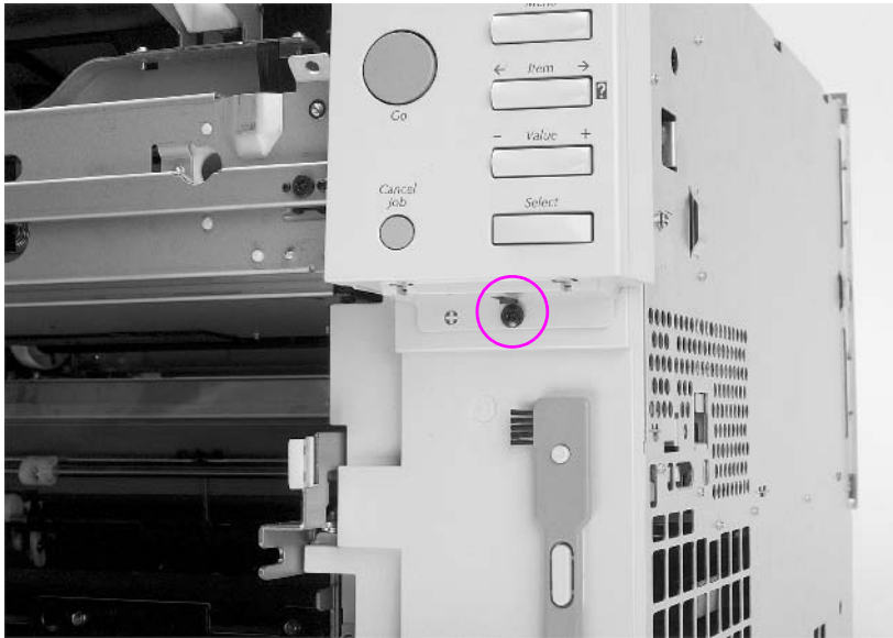
Figure 6-11 Control panel removal and replacement
