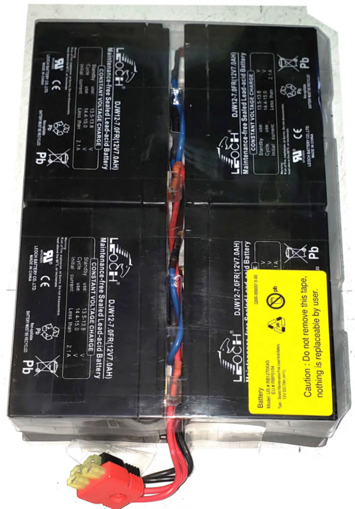
Completed Battery Cartridge
